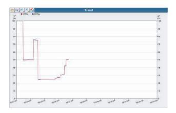
A deviation time out alarm occurs when the difference between the target position and the actual position exceeds the preset deviation alarm point (for more than the preset deviation time).
