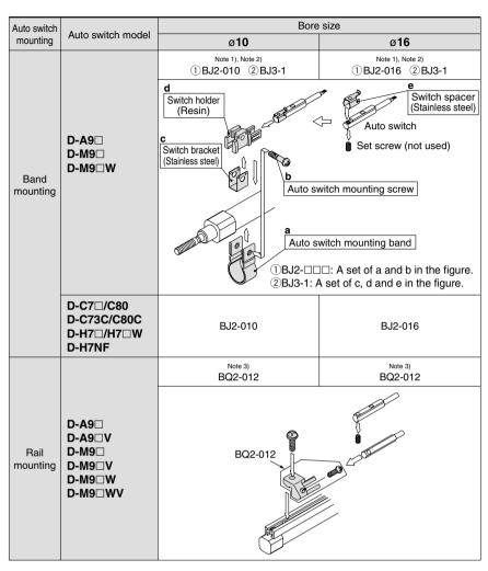
Note 1) Two kinds of auto switch mounting brackets are used as a set. Note 2) Auto switch mounting brackets are shipped together with cylinders. Note 3) When mounting a compact auto switch on the ø10 or ø16 rail mounting type, order auto switch
